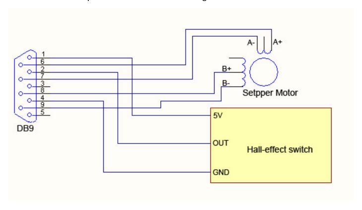
Input voltage of hall effect switch: 5V
